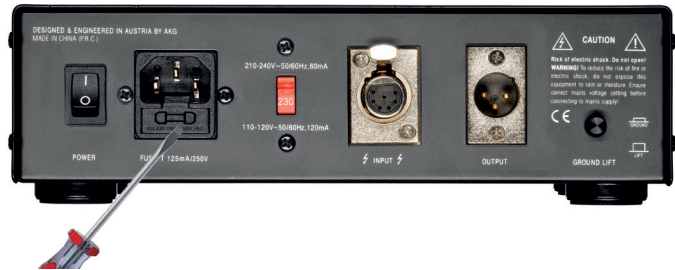
Figure 4: Opening the fuse compartment
