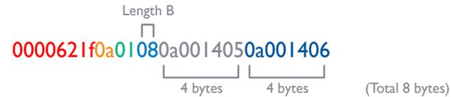
Length A includes Sub-option 1 (1-byte) and the Length B value (1-byte) plus the total of Length B (8-bytes). This makes the total 10-bytes which equates to 0a in hex.
