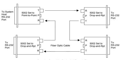
Operating Power May Be Applied Through The "P" Port or Through The DB-25 Connector Pins
