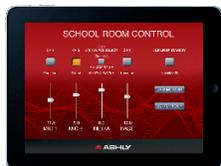
**11.9 Ashly Remote App for Apple iOS® Devices** A custom and secure touch-screen control surface for the iPad®, iPhone®, or iPod Touch® can be designed and deployed using the "Ashly Remote" application, available free on iTunes® or via the Ashly website. Controls, labels, and images are combined to manage key nXp amplifier functions over a wireless network connection.
