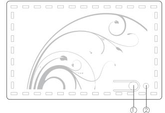
1. Timing button: Press this button once to show both input and output display resolution and while the OSD is still on the screen press it again to select output resolution from 1280x800, 1366x768, 1920x1200, 720p, 1080p 2. Power LED: This LED will illuminate when power is connected.
