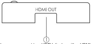
1. HDMI OUT: This slot is where you connect to a HDTV display with a HDMI cable for source signal display.
