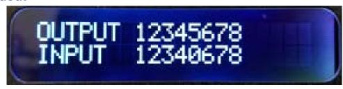
The LCD will reflect what Output is routed to which input when in an idle state.
