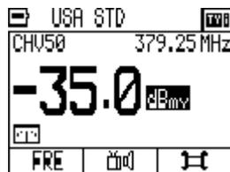
The unit will display the audio carrier frequency, the signal strength and play the audio.
