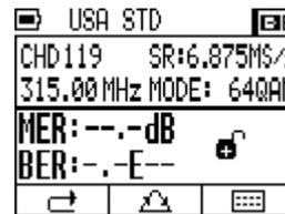
Press **F2** to enter the QAM measurement, as shown in Figure:
