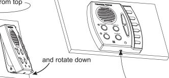
6. Tighten screw to lock in place
