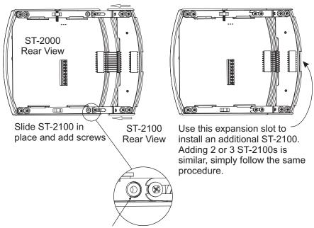
**IMPORTANT:** Hole in this bottom bracket must fit over plastic boss. (Metal must not sit on top of plastic. Or button functions may be affected.)
