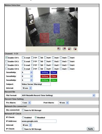
VIDEO SERVER supports three motion detection areas on each channel. When the motion is triggered, it can send out the video to a certain email address or upload the video to a FTP site. If the user has a SD Card, they can also do SD backup. The user can click on
