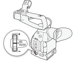
Turn the ND FILTER dial toward the + or - direction to select the desired ND filter setting.
