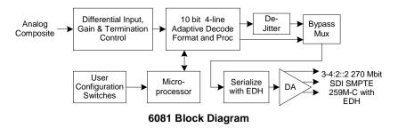
Features include user configurable 75-ohm input termination and user input gain control. The user has a choice of direct or de-jittered SDI output, Color Bar test pattern and Pedestal On/Off functions through externally accessible switches.
