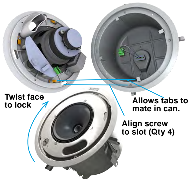
Figure 31. Four Twist-Assist™ face tabs inside the back can instantly secure the loudspeaker to the back can with a twist.
