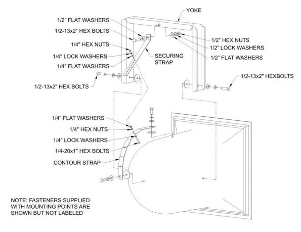
R2 YOKE ASSEMBLY: EXPLODED VIEW
