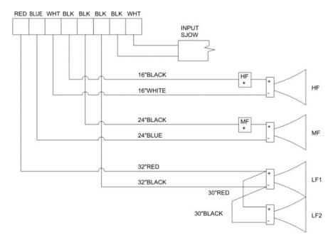
FIGURE 6: R2 Wiring (Models R2-474Z, R2-694Z, R2-77Z and R2-94Z)
