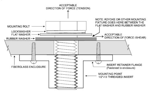
FIGURE 3: R2 Mounting Point Loading
