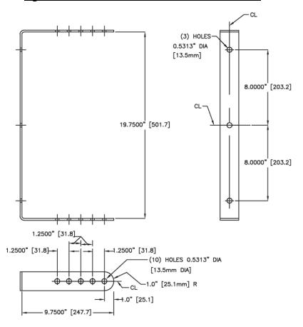
Figure 7 - W2-228 and W2-2W8 Yoke Assembly
