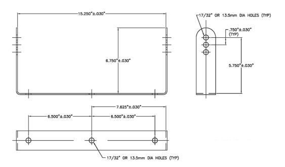
Figure 5 - W2-218 Yoke Assembly
