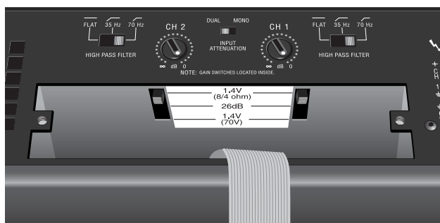
Figure 5.1 Input Sensitivity Switches for CTs 600/1200
