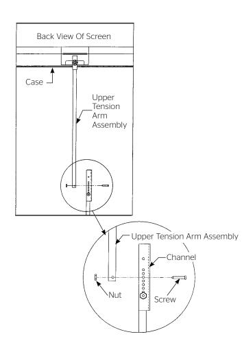
**NOTE:** Tensioning of the Deluxe Model B picture surface was made at the factory. Should more tension be required, the screw in the channel holding the upper tension arm assembly should be moved upward in holes allotted for this purpose. For any adjustment, it is recommended that the screen be removed, placed on a flat surface and a pair of pliers and a Phillips screwdriver be used in removing the screw and nut.
