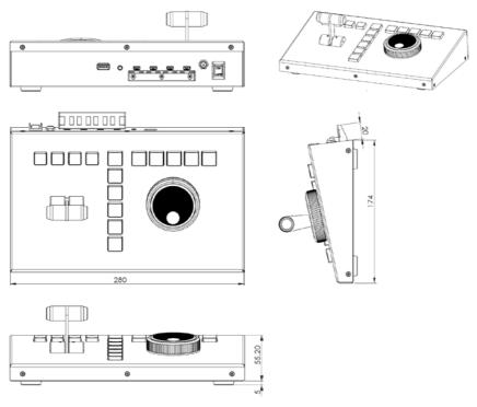
All measurements in millimeters (mm)
