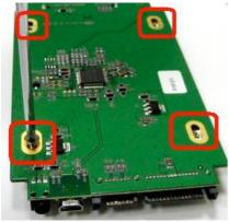
3. Push PCB into the HDD rack
