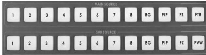
However, If we are only using the first four Composite inputs and one DVI input then switching becomes confusing. We want to avoid choosing the wrong buttons (5, 6 and 8) that have no video supplied to them. So re-assigning the video sources that we are using to the first five buttons of the Main and Sub Source rows can make switching easy. It can also make us less likely to press a wrong button that will result in no video or 'dead air'.
