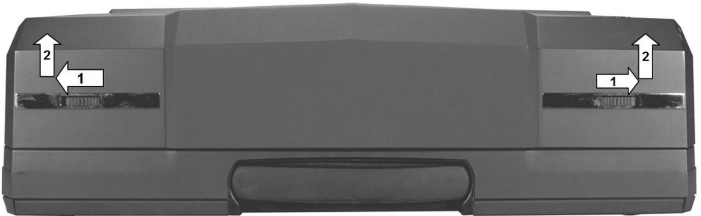
To open the HS-600 monitor lid slide the thumb catches in the direction shown to their outer most position. Then lift the monitor lid upwards away from the keyboard and carry handle.
