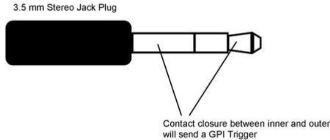
This GPI socket can also be used as a GPO socket to trigger record or playback events with other equipment such as the Datavideo DN-200, DN-400 or DN-500 recorders.
