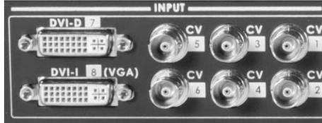
If we are using all of the video inputs then this numbering scheme works well and matches the default video assignments of the Main Source and Sub-Source rows of buttons on HS-600 keyboard.
