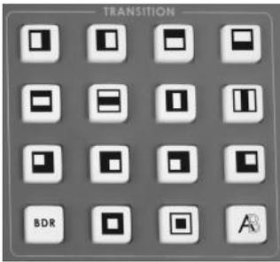
The HS-600 features 14 programmable wipe patterns and an A/B dissolve or fade.
