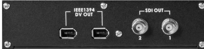
The two DV25 outputs carry audio as well as video. The DV output can be connected to a DV25 deck or recorder such as the Datavideo DN-60, DN-200, DN-400 or DN-500. Alternatively you could also connect this DV output to a computer DV capture card.
