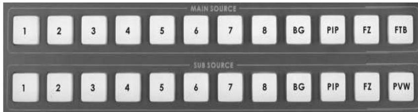
The Sub Source Row is the Cued channel; this channel will appear in the PST or Preview window. The Sub Source selection determines which input will be transitioned to when using any of the transition controls.
