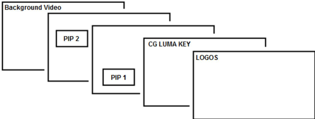
The **Background video layer** is the normal video layer when mixing and switching with the HS-600. It occupies the whole screen area of the Program output. This layer can be hidden or part hidden by the PIP, LUMA KEY and LOGO layers in front of it.
