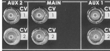
These outputs should remain set in the menu as two Composite (CV) outputs and a single Y/C output.
