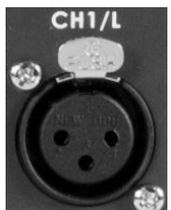
The HS-600 has two balanced XLR input connectors, each with 3 pins. These XLR inputs are associated with the Line and Mic Switch as well as the Phantom power switch. These inputs can be used to supply a stereo input (maybe the output of a larger audio mixing desk) or two separate mono audio channels left (L/CH1) and right (R/CH2) for microphones.
