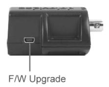
This unit allows you to operate the functions of the camera up to 300m away with the MCU-200S unit.
