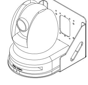
SLIDE CAMERA WITH MOUNTING BASE IN POSITION OVER THE MOUNTING PLATE SLOTS. SECURE (3) PLACES USING SCREWS SHIPPED WITH CAMERA MARKED "A"
