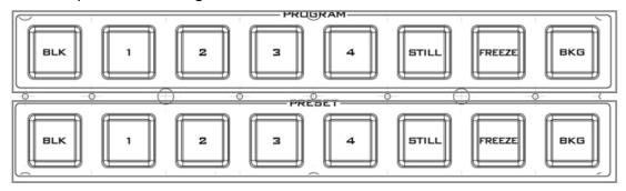
2. Select the next source on the Preset row of buttons and then press the **CUT** button.
