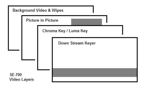
The **background video layer** is used for transitioning between Preview and Program sources. This layer also includes any selected wipe transitions. This layer can be hidden or hidden in part by the PiP, Keyer or DSK video layers in front of it.
