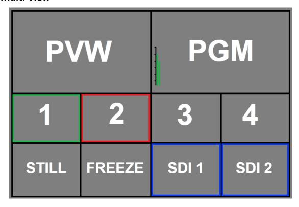
The SE-700 Multi view output can be supplied from the HDMI or SDI outputs, see Chapter 3. The layout of the multi view cannot be changed. The sources can be swapped around using the cross point section of the Inputs menu.
