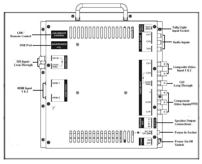
**LAN Remote Control:** Use a crossover Ethernet cable for direct connection between TLM-170P and the PC RJ-45 port. See *Remote Control Setup section* for more details.
