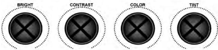
Individual adjustments for Brightness, Contrast, Color and Tint (Tint is for NTSC only). These four adjustments can be adjusted with a X headed screwdriver. It is recommended that you use a Test Pattern to adjust the monitors.
