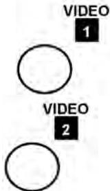
Composite Video Input 1 – Connect a composite video signal to here. The TLM-700 will auto detect whether the signal is NTSC or PAL.
