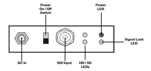
**HD / SD LEDs -** Once a signal has been detected the appropriate LED will light to indicate format.
