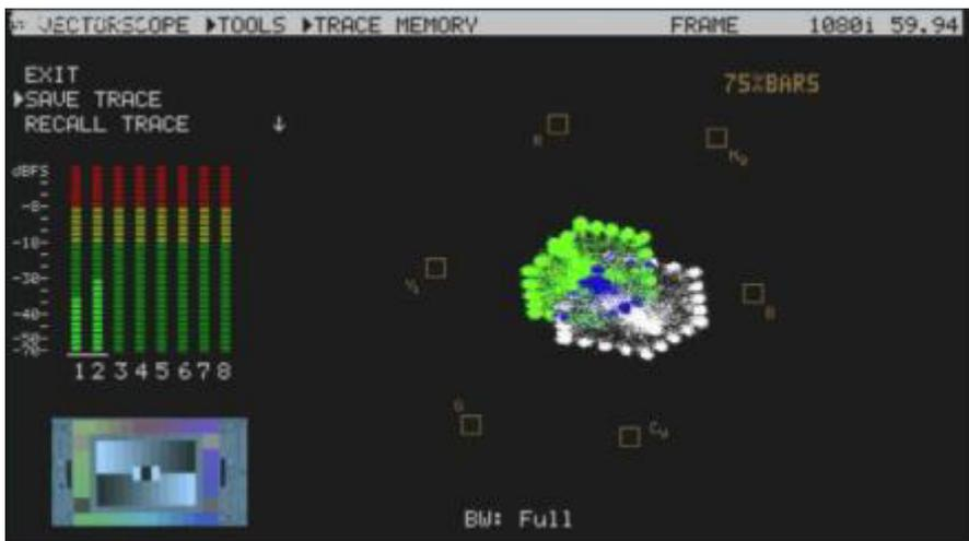
4. Feeding camera output of 75% colour bars into a Video Switcher confirms if the colour image is correct after the switcher too.
