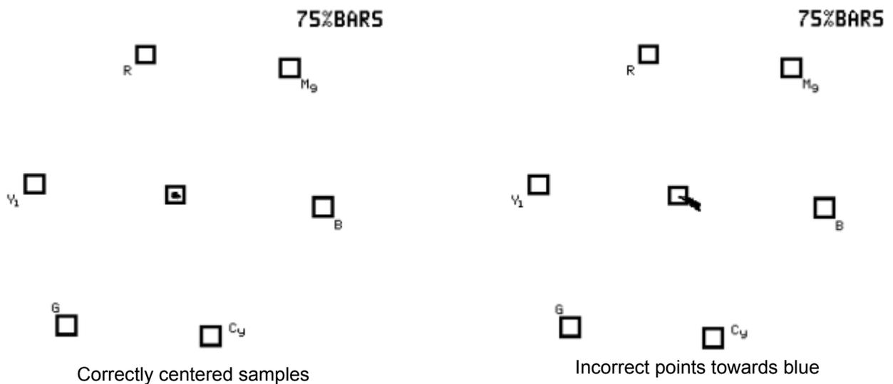
6. Once white balancing is complete cap the camera lens to produce black video. The sample points should only appear in the same center graticule box of the VSM-200 Vectorscope
