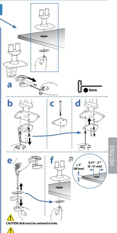
CAUTION: For secure arm attachment and to avoid equipment damage, plate must make contact with underside of desk on both sides of the hole.
