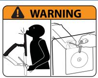
WARNING! Stored Energy Hazard: The arm mechanism is under tension and will move up rapidly, on its own, as soon as attached equipment is removed. For this reason, DO NOT remove equipment unless the arm has been moved to the highest position! Failure to follow this instruction may result in serious personal injury and/or equipment damage!
