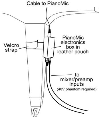
Figures 16. Attaching the Pouch to the Piano Leg.
