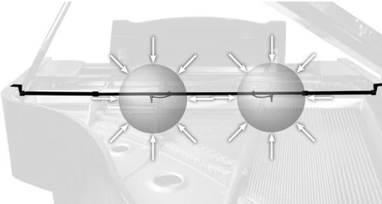
Figure 3. Random Incidence Microphones inside a piano pick up sound accurately from all directions
