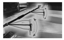
Figure 12. Adjusting the Microphone Height
