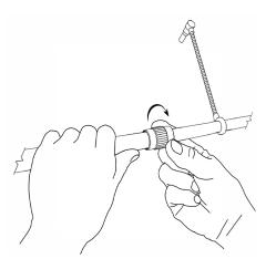
Figure 4. Loosening the Clutches
