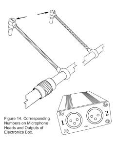
12. Notice in Figure 14 that the top of each microphone head has a number. These numbers correspond to the numbers on the rear of the electronics box. Depending upon how the PianoMic<sup>TM</sup> is placed in the piano the high strings will be indicated by either the number 1 or number 2. Once the PianoMic™ has been placed, identify the microphone numbers on the mic heads for both the high and low strings and remember that they correspond to the numbers on the rear of the
