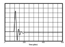
Fig. 3. Impulse Response (Typical) of SR40
