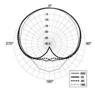
Fig. 4. Polar Response (Typical) of SR40
