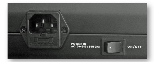
On the back of the MIDICON PRO™ you will find the AC mains connector with fuse (1A slow blow) and the power ON/OFF switch. The power supply is compatible with both USA and Europe (100-240V).
