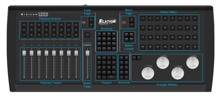
**PLAYBACKS:** This includes most of the left side of the control panel; (8) touch sensitive and motorized playback faders with (3) buttons above each fader along with page select buttons and a page display.
