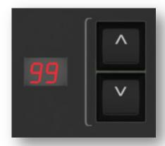
There are (2) separate page controls, one for the playbacks and another for the matrix buttons. Paging essentially gives you additional sets of faders and matrix buttons to work with. Paging can be controlled by either your lighting software or the **MIDICON PRO**<sup>™</sup>. If your software can control the paging you can have up to (99) pages to work with.
