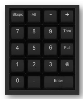
In the middle of the panel is a lighting control style numeric keypad for data entry. Your lighting software will determine the behavior of these keys if it supports the **MIDICON PRO™** directly, otherwise you will have to link each button to a function using the setup menu in your lighting software. Please refer to the **MIDI MESSAGES** section at the end of this manual for each button's default MIDI Note message.
