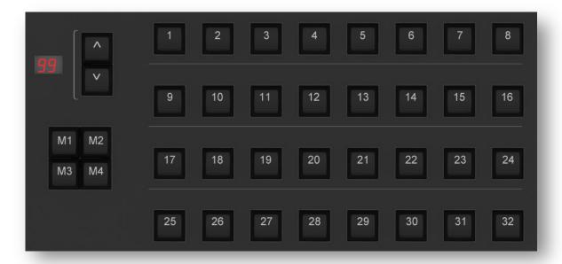
These (32) buttons are used to call lighting effects, scenes, colors, etc. If your lighting software does not directly support the **MIDICON PRO**<sup>TM</sup> you will have to link each button to a function using the setup menu in your lighting software. Please refer to your lighting software's manual for instructions, as this will be different for each program.
