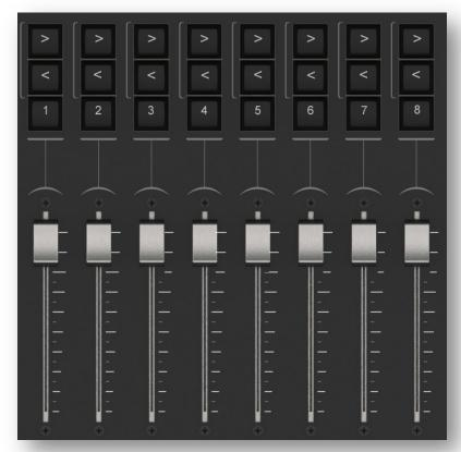
The playback section was designed to take advantage of the playback features in most lighting software programs where a playback fader and some associated buttons are used. There are **FORWARD**, **REVERSE** and **BUMP** buttons above each playback fader. The function of each button will vary depending on the software that you are using. The playback faders are touch sensitive and motorized.
