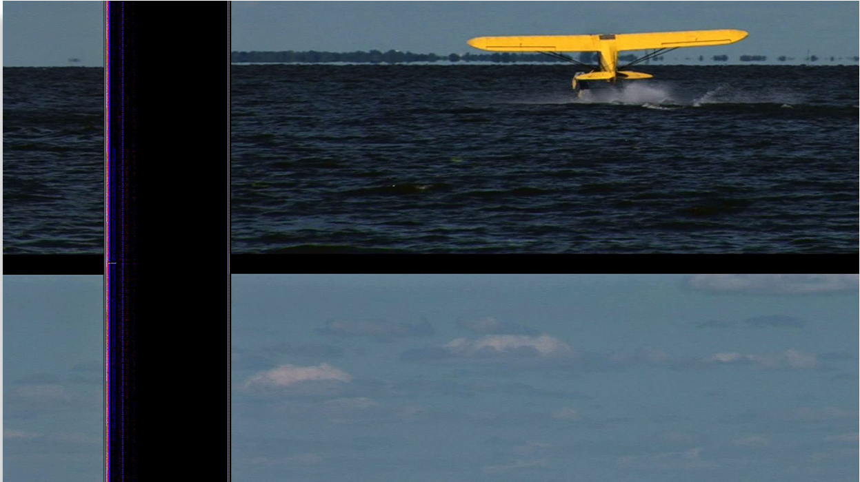
HDMI monitor output example illustrating Horizontal shift. H and V shift enables inspection of content in the horizontal and vertical intervals.
