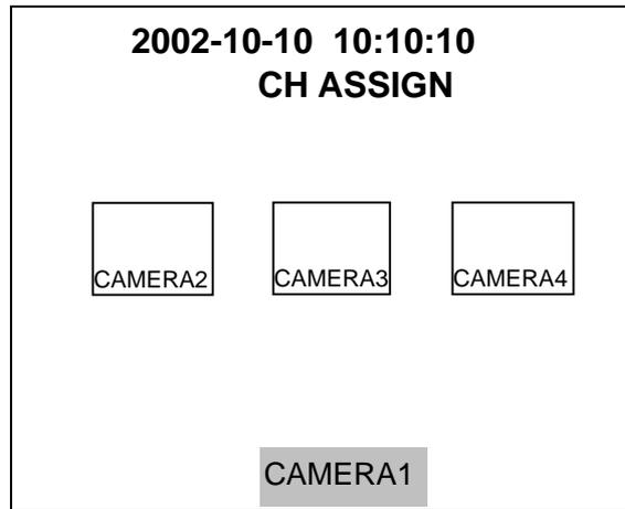
Factory default P-in-P3 channel assignment is shown above for example. Title flashing screen channel can only be assigned (hatched in the figure above). The table below shows how to assign channels.
