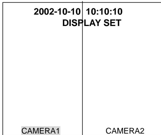
When in V2, H2, V3 or H3 mode, only half sized screen view can be adjusted by tilt up/down or pan left/right. Also when in V2 or H2 mode, only the title flashing screen view can be adjusted. Factory default screen view settings are shown below.
