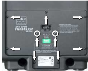
TV8 (x7 small Screws) (x2 med. Screws Circled)
