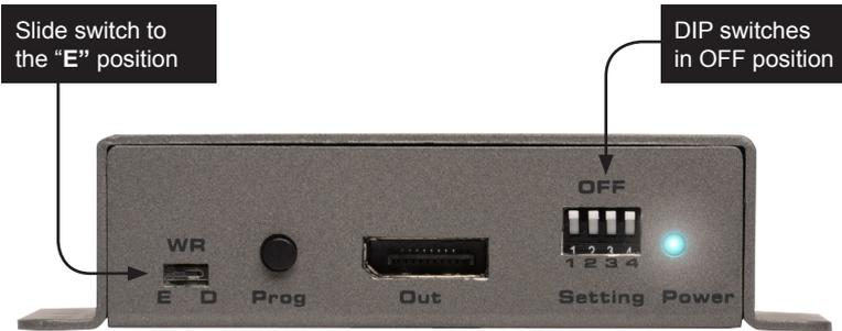
5. Connect the included 5V DC power supply to the detective. The **Power** LED will glow bright blue if the sink device contains a valid EDID. If the EDID is corrupt or invalid, then the **Power** LED will glow bright red.
