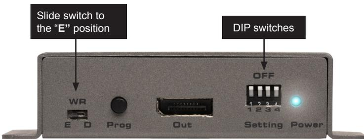
3. Set the **WR** (write) switch to the “**E**” position in order to allow the EDID to be written to the local input.
