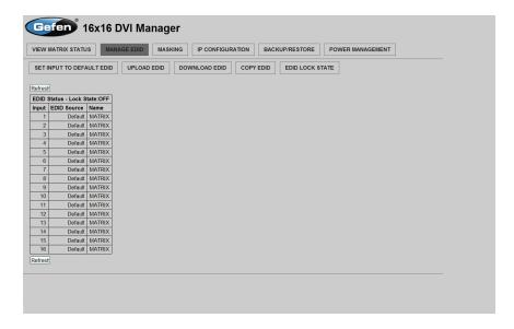
The **Manage EDID** page is used to see the status of the EDID saved in the local storage location for each input. This section has additional tabs for advanced EDID functions. These tabs are:
