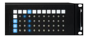
The button for Input 3 will glow blue momentarily and each LED will change from Input 1 to Input 3.
