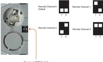
Exposed DIP Switch bank between the battery chambers.
