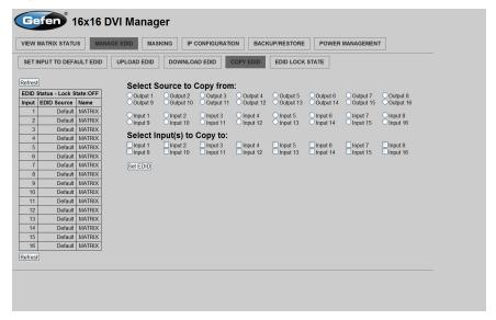
On this page, the user can select an EDID from either the local memory locations (Input) or from a monitor that is currently attached to any output and copy that EDID to any other LOCAL memory location. This will permits control of what EDID information will be passed to each source connected to the 10x4 DVI Dual Link Matrix.
