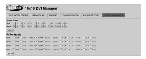
The **Power Management** page is used to set optional +5V power on an input to power specific optional devices. The current status of this feature for each input can be viewed on this page. To set this feature for each input follow the steps below.
