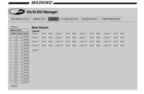
The **Masking** page is used to hide an output from displaying any video. From this page, all outputs can be set to "Active" or "Mask". When an output is set to "Active", it will function normally. When an output is set to "Mask", it will not output any video. To set the "Active" or "Mask" mode, follow the steps below.
