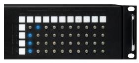
The Input 2 and for Output 1 buttons will turn off. The source connected to Input 2 should now be displayed on the monitor connected to Output 1.
