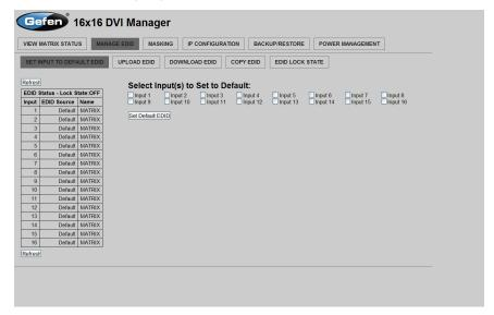
On this page, local memory locations can be selected to receive the built-in EDID stored in the 10x4 DVI Dual Link Matrix. To set an input's local memory location to the default EDID follow the steps below.
