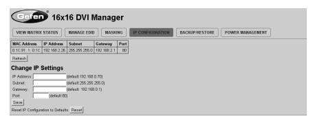
The **IP Configuration** page is used to set the IP settings that will be used to access the Web interface. The following items can be configured from this menu.
