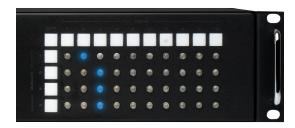
In the example above, Input 3 has been routed to Outputs 2, 3, and 4. From the previous example (see page 9), Input 2 has been routed to Output 1.
