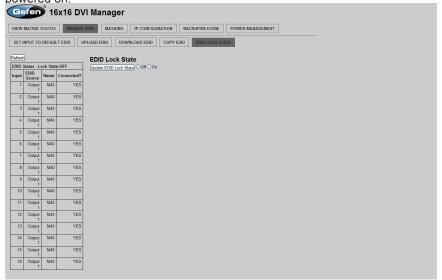
The EDID Lock State can be enabled (ON) or disabled (OFF). The EDID Lock State is used.
