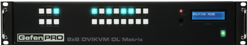
4. Select the desired input (source) button (1 - 8). For this example, we will route the source connected to Input 6 to each of the outputs in step 3. Therefore, press button **6** on the bottom row. The selected input will glow bright blue.
