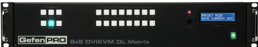
The LCD will indicate that the matrix is in *save preset mode*:
