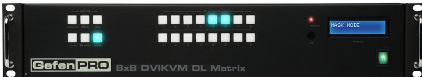
3. Press the **Set** button to mask the selected outputs. The **Set** button will flash momentarily.
