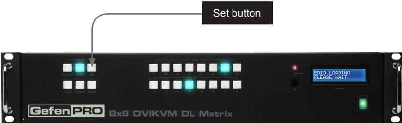
5. Once the **Set** button is pressed, the matrix will begin copying the downstream EDID from the display (or other sink) to the EDID from the selected output to the specified input.
