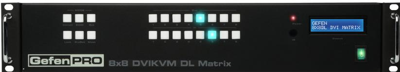
If Output button **1** or **3** is pressed, the button for Input 6 will also be selected.
