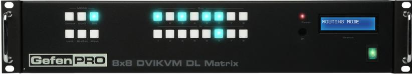
5. Press the **Set** button on the front panel, once again. Pressing the **Set** button again tells the matrix that we have completed the routing operation. Once the **Set** button has been pressed, the LCD will indicate that the routing process has been completed.
