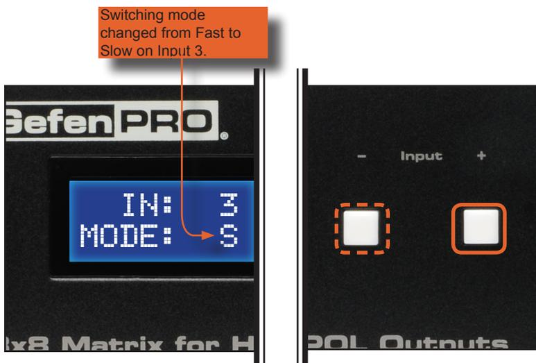
To change the switching mode of another input, press the **Output +** or **Output -** button to navigate to the desired input. Press the **Input +** or **Input -** button to toggle the switching mode between Fast (F) or Slow (S).
