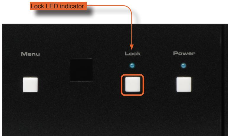
The Lock LED will glow bright blue to indicate that the front-panel buttons on the 8x8 Matrix for HDMI w/4 ELR-POL Outputs have been locked.
