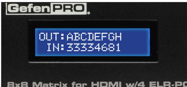
If all inputs are routed to their respective outputs, the front-panel display will appear as follows:
