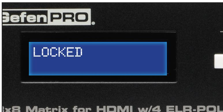
2. To unlock the 8x8 Matrix for HDMI w/4 ELR-POL Outputs, press the **Lock** button a second time.
