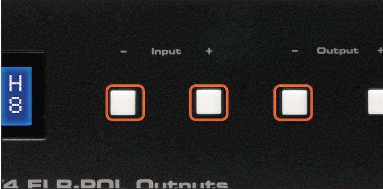
2. Use the **Input +** (or **Input -**) button to change the IR channel. Press the **Input -** button to decrease the IR channel value. Press the **Input +** button to increase the IR channel value.
