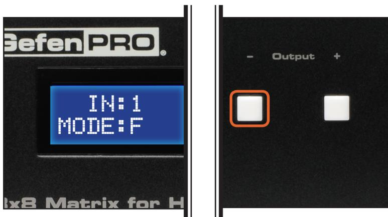
The letter **F** indicates that the HDMI input is using Fast Mode switching. If the HDMI input is set to Slow Mode switching, a letter **S** will be displayed under the input.
