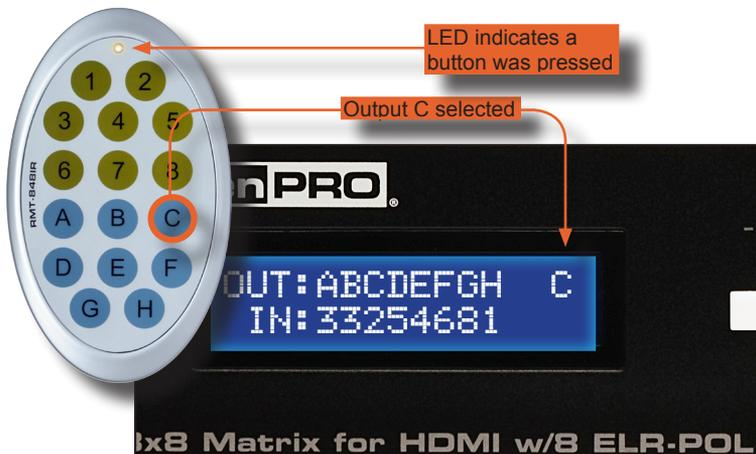
2. Select Input 4 by pressing button **4** on the IR Remote Control. The number 4 will appear in the lower right-hand corner of the LCD display:
