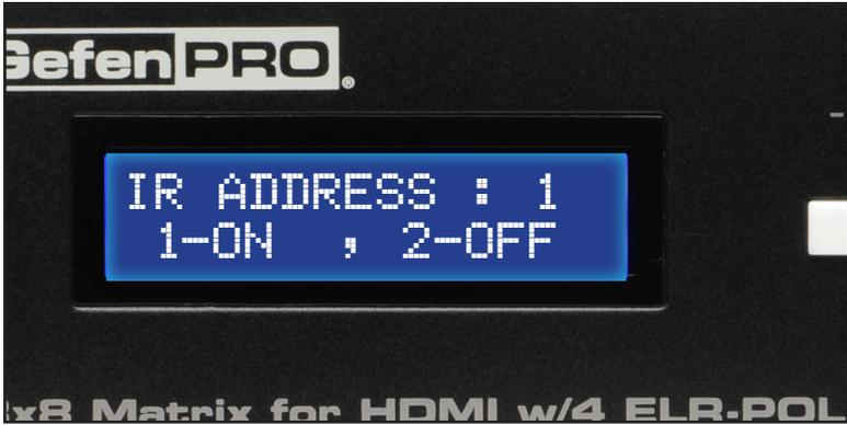
In this case, the 8x8 Matrix for HDMI w/4 ELR-POL Outputs is set to IR channel 1. Therefore, DIP switch 1 on the IR Remote Control must be set to the ON position and DIP switch 2 must be set to the OFF position.
