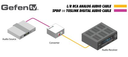
Wiring Diagram for the Digital Audio to Analog Adapter
