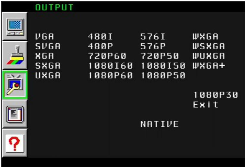
This menu sets the output resolution for all video sources. The OUTPUT button on the IR remote control unit also cycles through each of these available resolutions.
