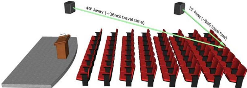
The AD-340 Audio Delay Processor is designed to provide a flexible way to adjust for these types of delay by adding a digital delay function based on 5 different delay types.
