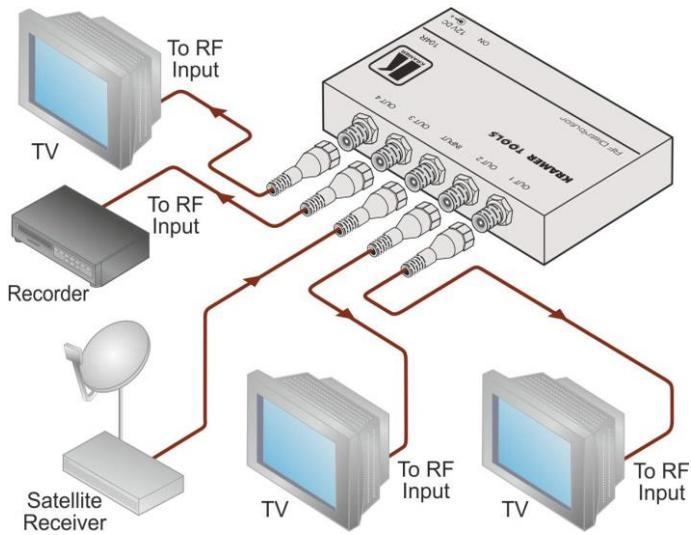
Figure 2: Connecting the 104R RF Distribution Amplifier
