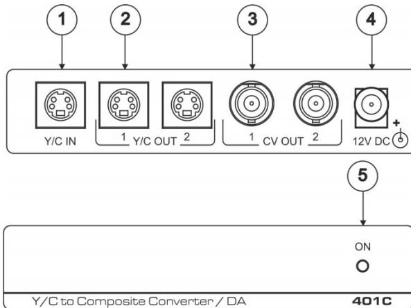
Figure 1: 401C Y/C to Composite Converter/DA
