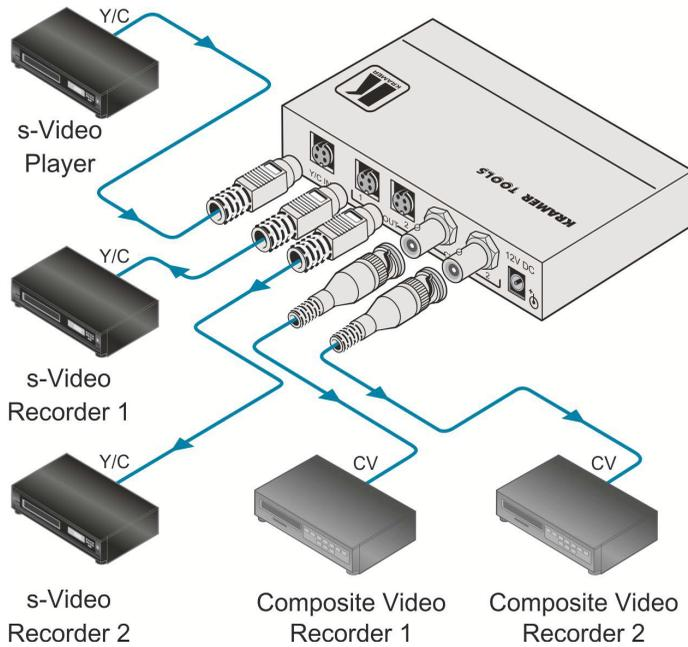
Figure 3: Connecting the 401C
