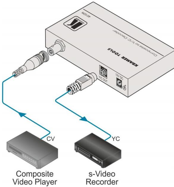
Figure 4: Connecting the 401DN
