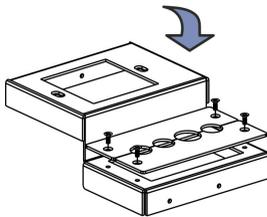
Mount the Inner Frame into the **TBUS-3xl** enclosure.
