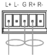
Figure 4: Connecting the Unbalanced Stereo Audio Output
