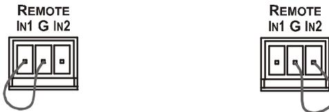
Figure 3: Connecting the REMOTE Input Select Connector
