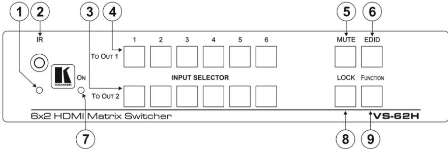
Figure 1: VS-62H 6x2 HDMI Matrix Switcher Front Panel
