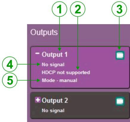
Figure 13: The Output Buttons
