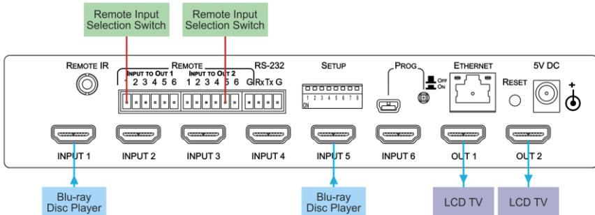
Always use Kramer high-performance cables for connecting AV equipment to the VS-62H.
