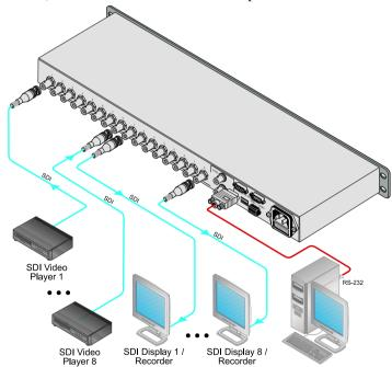
Figure 6: Connecting the SD-5788V
