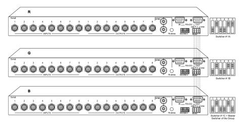
Figure 11: Component Switcher: VS-88V Group Connection
