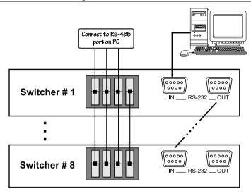
Figure 10: System Connection: Switchers and the PC
