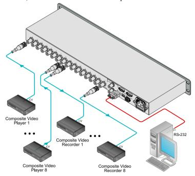
Figure 5: Connecting the VS-88V
