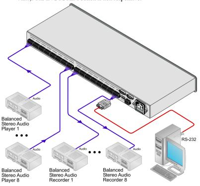
Figure 4: Connecting the VS-88A
