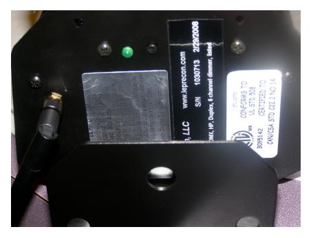
The LED located on the dimmer endplate shows the status of the wireless link.
